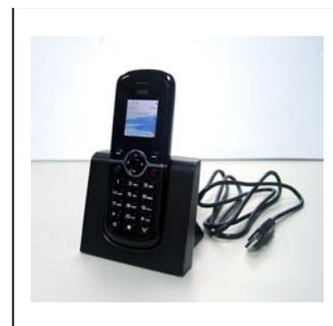
WP589 is a WiFi client handheld SIP IP phone with color LCD display and Slim, Compact design. It links to IP network through WiFi AP which complies with IEEE 802.11 b/g standard. It is suitable for Internet Telephony Service provider, Office IP-PBX or home use Wireless phone.
