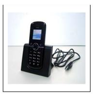
WP589 is a WiFi client handheld SIP IP phone with color LCD display and Slim, Compact design. It links to IP network through WiFi AP which complies with IEEE 802.11 b/g standard. It is suitable for Internet Telephony Service provider, Office IP-PBX or home use Wireless phone.
