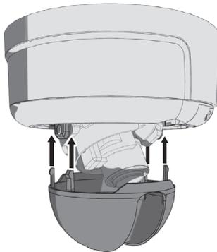
**Figure 8.** Installing the Dome Liner
